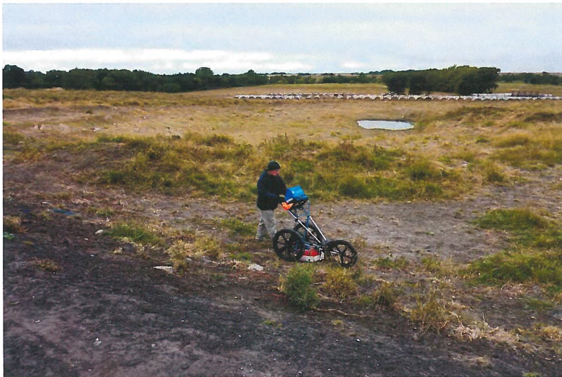
GPR data collection using the GSSI Utility Scan System in the buffalo pasture near the excavated area and stock pond.
